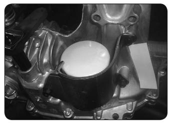
The check plug is located at the top center of the inside case of each transaxle. The transaxle can be filled with oil by removing these check plugs from both transaxles and pouring the oil in the hydro overflow tank, located behind the seat. Oil will begin to run out of the check plug holes when the transaxles are full. Use only 20w50 motor oil in the hydro system.
